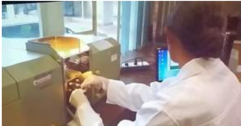
Figure 5.3. Mineral analysis of feed samples using Atomic Absorption Technique
